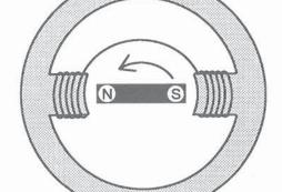
In electric generating stations alternating electric current is produced when a magnet spins within a coil of wire.
