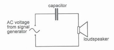
Since the loudspeaker is a combination of both inductance and resistance, the circuit shown is actually a combination of inductance, capacitance and resistance (i.e. a series LCR circuit).
